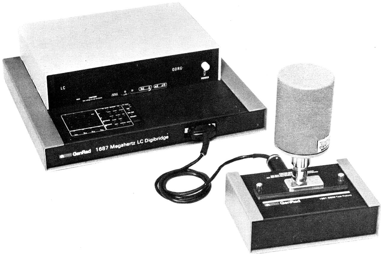
Figure 3-9. Calibration setup. The coaxial capacitance standard is shown on the reference-standard adaptor, on the test fixture.
