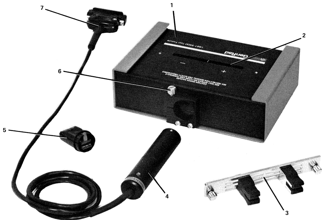
Figure 3-1. Test fixture and accessories. 1 – Test fixture; see Table 1-3. 2 – Pair of slots for radial-lead DUT, labeled with polarity of bias, if any. 3 – Axial-lead adaptor. 4 – Probe and cable assembly, shown in position for plugging into test fixture. 5 – Probe nose, shown unplugged from probe. 6 – Thumb screw used to tighten clamp that holds probe securely in position. 7 – Connector that fits J8 on the front of the Digibridge.
