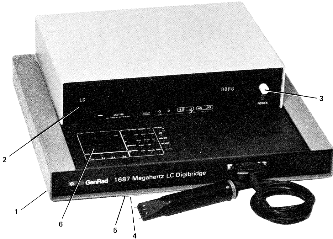
Figure 6-1. Front view, showing replaceable mechanical parts.
